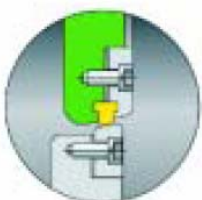
Fig.6 Rubber seal(Replacement seat)
