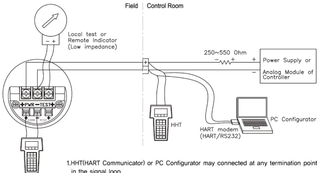
1. HHT(HART Communicator) or PC Configurator may connected at any termination point in the signal loop.
