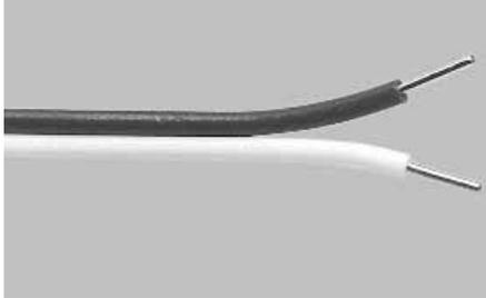
The SERIES 505 is the most economical wire produced. Unlike some competitive "ripcord" type constructions which use only a stripe to establish polarity, SERIES 505 single conductors are fully color coded. The conductors are individually insulated with the proper colored PVC and fused into "ripcord" using a proprietary process.
