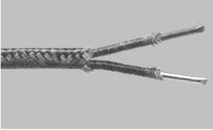
SERIES 305 is specifically constructed for light duty applications where size is a critical factor. The single conductors are insulated using a specialized yarn wrapped on the conductors in layers. This yarn is then impregnated to add abrasion resistance and enhance electrical properties. The insulated single conductors are then laid parallel and covered with a layer of braided glass. A final impregnation is applied to the braid.
